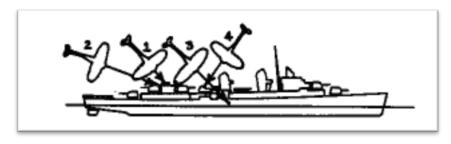
Struck amidships by four Japanese suicide planes with bomb loads. Minor fires. Deck, bulkheads, shell plating demolished in way of three after machinery spaces. Three after
